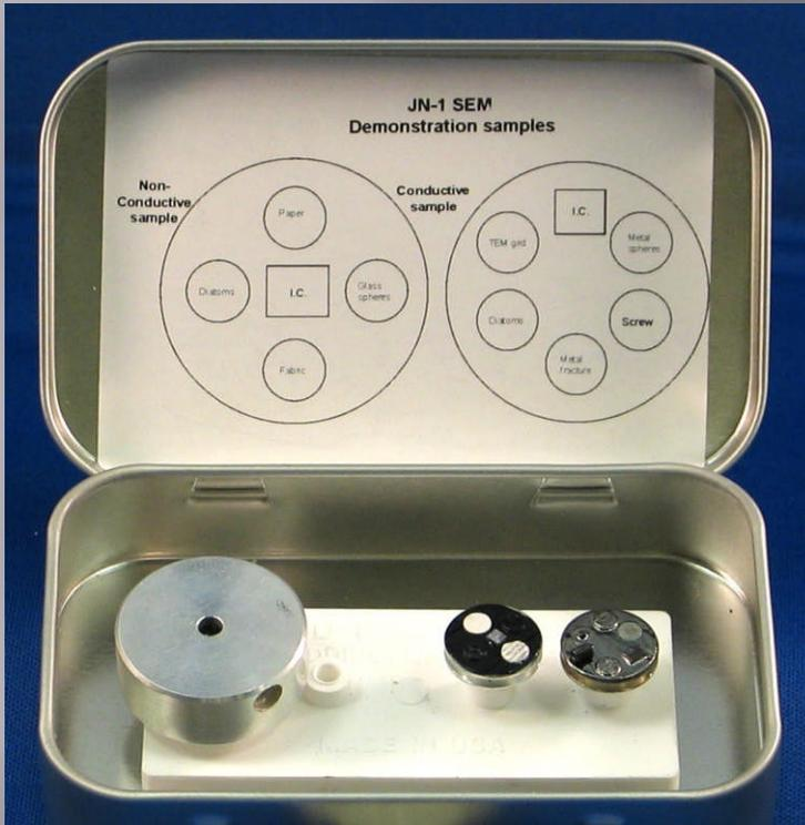
One stub has six **conductive** samples consisting of an integrated circuit chip, metal spheres, a set screw, ductile metal fracture, diatoms and a TEM grid. The entire stub surface is coated with about 20nm of Au:Pd.
