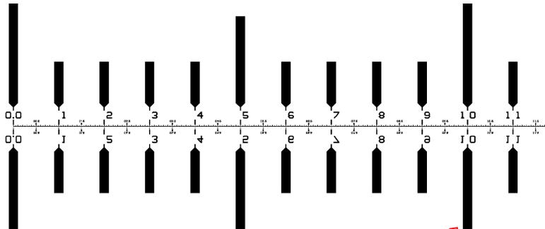
Markings are all on one side. Mirror image markings are provided so right reading numbers are always seen.
