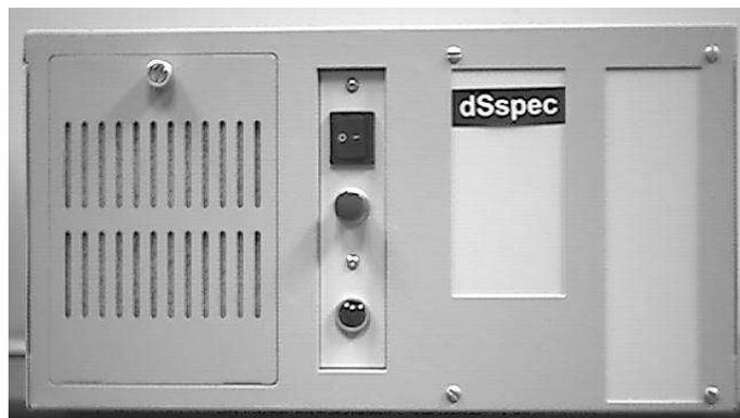
**dSspec7** is housed in a 13" X 16" X 7" cabinet. Normally placed near the instrument's column, no rack mounting or further cabinetry is required. An emergency power off switch and power indication lamp is located on the front.
